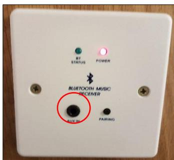
To connect a device via an AUX cable, plug one end of the cable into the 'headphone socket' of the device and the other end into the hole labelled 'AUX in' on the Bluetooth panel on the left-hand side of the sound system box. Use the 'Bluetooth Receiver' dial on the front of the box to control the volume.
